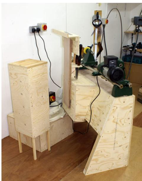
Back of lathe stand with sack of cement enclosed in box (tool and calliper stand attached).
