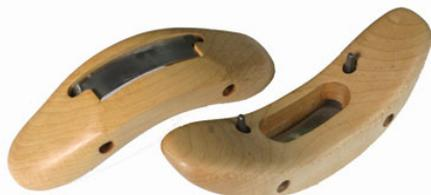
The key differences are that the shavings emerge from the top of the tool through a generous slot, and the back of the tool is solid wood, giving a much wider area for the thumbs which do almost all of the work. The tool is also not as tall as its predecessor, which makes it easier to hold for those with smaller hands.
