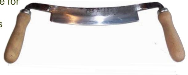
The blade has been forged from spring steel, and maintains a razor sharp edge over a long period.
