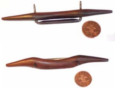
**Small Spokeshave:** This tiny tool has transformed the making of Windsor chairs. It is crucial to the shaping and finishing of spindles, and is also used on the bow, and for fine work on the seat. The blade is easily sharpened, and is adjusted by tapping the tangs with a small hammer. The excellent steel keeps its edge for at least one chair, before requiring resharpener.
