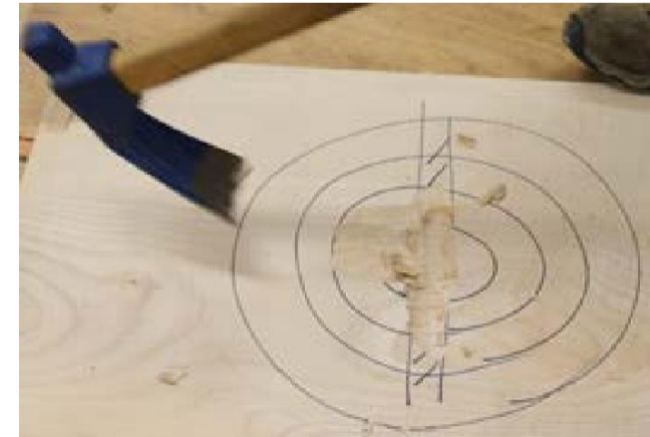
Chopping down towards the target trench (Pic.3, above), which is then done from the other side, until the adze removes the waste (Pic.4, right)
