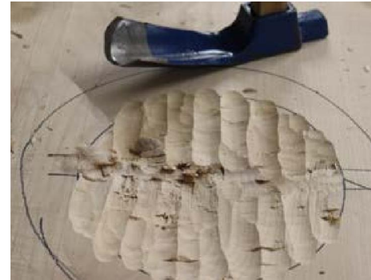
Chopping down towards the target trench (Pic.3, above), which is then done from the other side, until the adze removes the waste (Pic.4, right)
