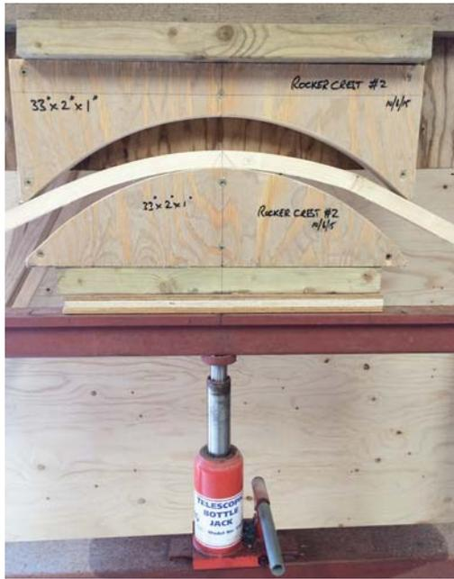
bend successfully. Otherwise, the wood should not be dry. In my experience you can cut down an oak tree and bend the wood five minutes later, but ash does not like that. Ash bends better when air dried. I store my ash for bending as 1 1/4in thick boards under cover, but in an open-fronted shed. The moisture content stabilises at around 20% and the wood will remain bendable for years.
